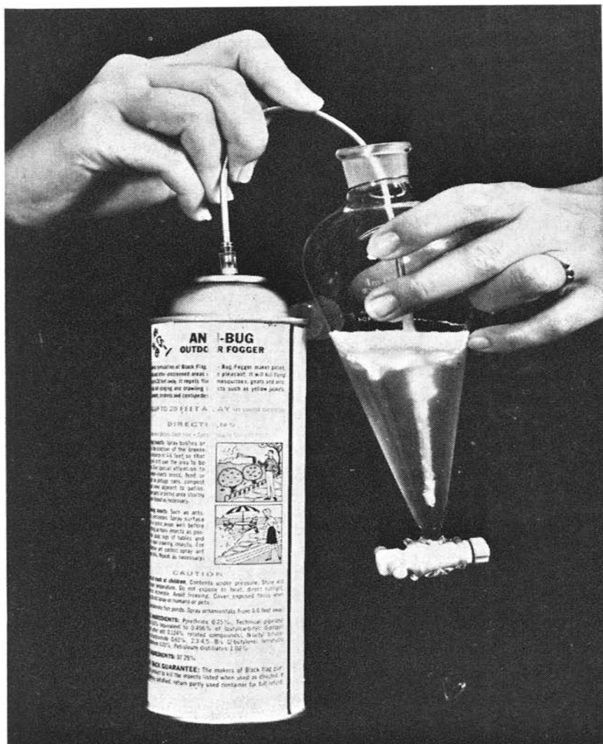
Fig. 3. Example of sampling aerosol container for sample analysis.
